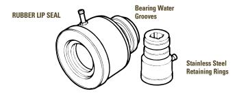
Another common type of mechanical seal used on rotating propeller shafting is the lip seal. Lip seals are similar to stuffing boxes in that they utilize the propeller shaft as a sealing surface. A rubber ring with a lip on the inside diameter fits over the propeller shaft. The tight interference fit between the rubber lip and the propeller shaft ensures continuous contact and creates a seal.
